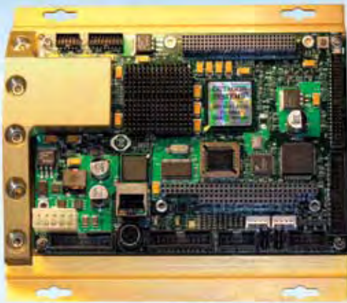
EPIC™ XE-900 CPU, with conductive cooling system
