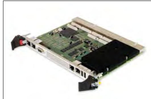
CR11 - CPC16U SBC with Intel Core Duo Processor
