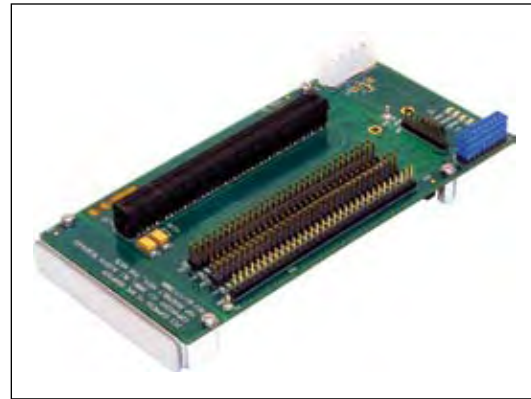
Adapts PCIe card to an XMC site.
