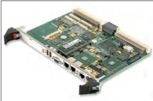
V7865 - VME6U SBC with Intel Core Duo Processor
